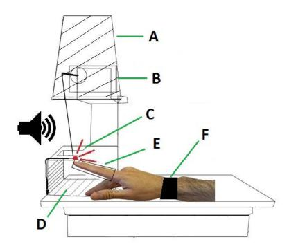
Fig.1. Sketch of the finger lifting device. A – opaque casing, B – servo drive, C – upper contact plate with LED, D – lower contact plate, E – metallic holder for index finger (here, shown transparent for clarity), F – strap for fixation of participant's hand.
